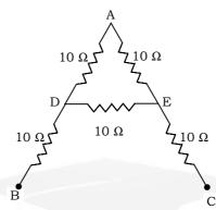
Find the net resistance between points B and C in the combination of resistances as shown in figure.
