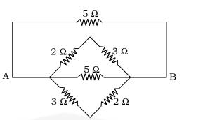
Calculate the equivalent resistance between the points A and B in the given Figure.
