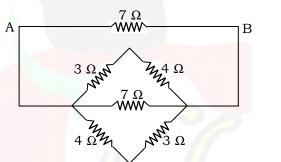
Calculate the equivalent resistance between the points A and B in the given Figure.
