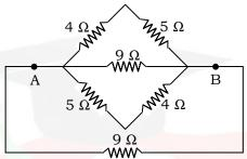
Calculate the equivalent resistance between the points *A* and *B* in the given Figure.
