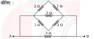
Calculate the equivalent resistance between the points A and B in the given Figure :
