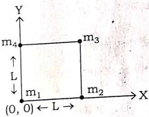
Particles of masses  $m_1 = 2$  g,  $m_2 = 2$  g,  $m_3 = 1$  g  $\overline{a}$   $m_4 = 1$  g are placed at the corners of a square of side L, as shown. Find the centre of mass of the system with respect to  $m_1$ .
