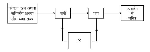
Write the name of X in the given block diagram of electric power plant.
