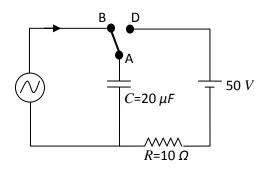
(A) Magnitude of the maximum charge on the capacitor before  $t = \frac{7\pi}{6\omega}$  is  $1 \times 10^{-3}C$ . (B) The current in the left part of the circuit just before  $t = \frac{7\pi}{6\omega}$  is clockwise.
