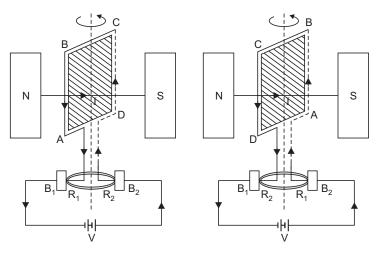
Working: As the armature coil is rotated in the mag. field angle  $\theta$  b/w field and normal to the coil changes continuously. An emf is induced in the coil. The direction of induced current is shown in figure.
